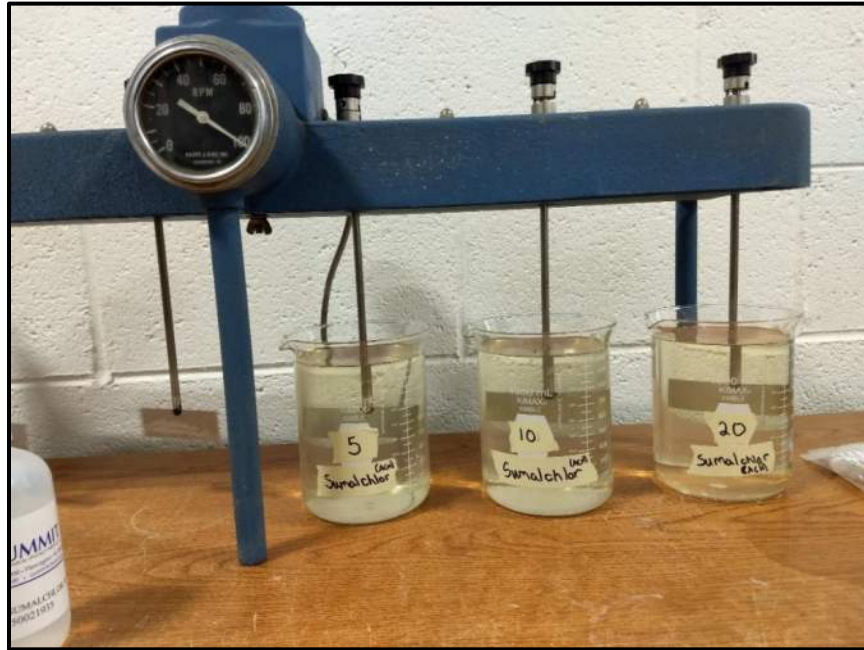
Figure 5. ACH Bench Testing
